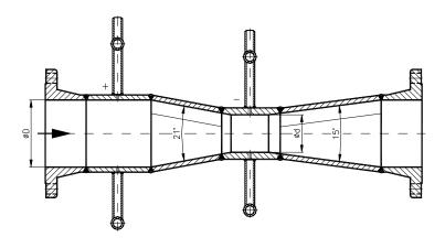
to be welded into the pipe; with a machained convergent section; 4 pressure bore holes with a ring chamber
