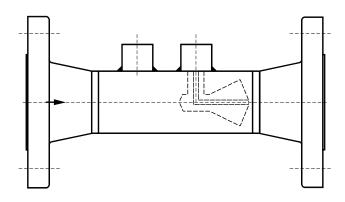
outside tapping connection through the support strut of the cone to the downstream face of the cone element. Generally, we provide cone meters with end flanges for easy mounting.
