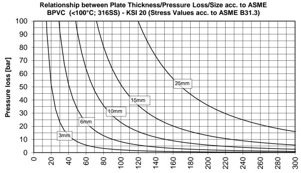
Internal diameter of the gasket between flange/plate [mm]
