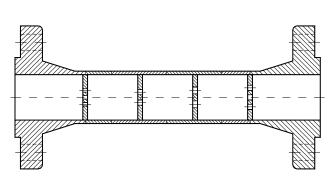
single step/hole restriction orifice
