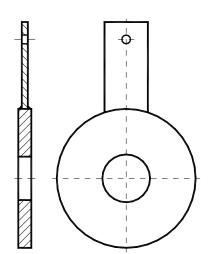
If the plant dictates limits to the noise level or if the pressure loss could lead to cavitation, an option is to use a multihole or multistage restriction orifice. A combination of multihole and multistage design is also possible. For most materials we also offer various hardness coatings of the orifice bore hole in order to achieve a higher durability and a longer service life time.
